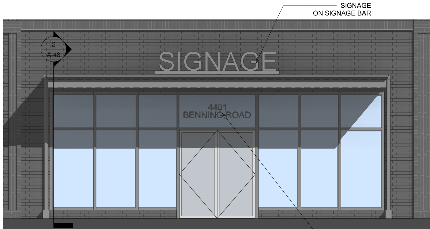
3 ENLARGED ELEVATION SIGNAGE 1/4" = 1'-0"
